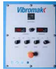
Electric Control Panel Elektrik Panosu
